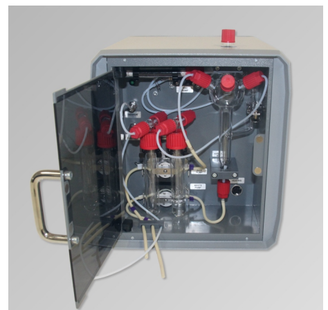
Interior view of H 2 S ANALYZER Cubi
